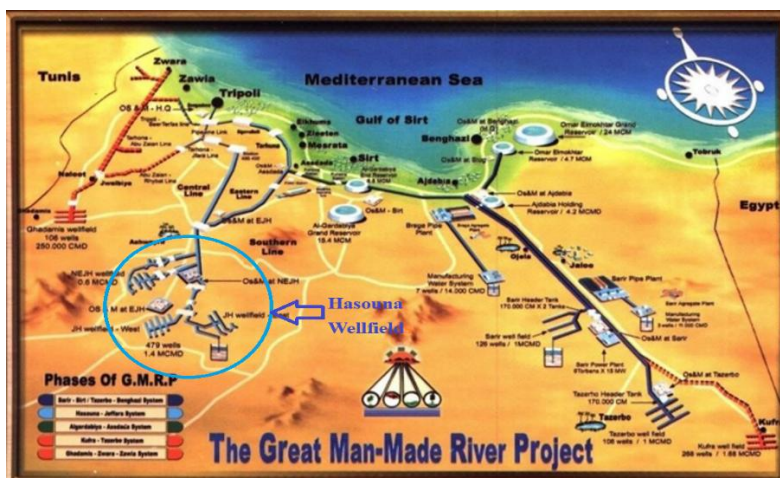
Fig. 1.: Layout of the Major Systems of the Great Man-Made river Project, showing the Hasouna Wellfields. (after MMRP, 2004)
